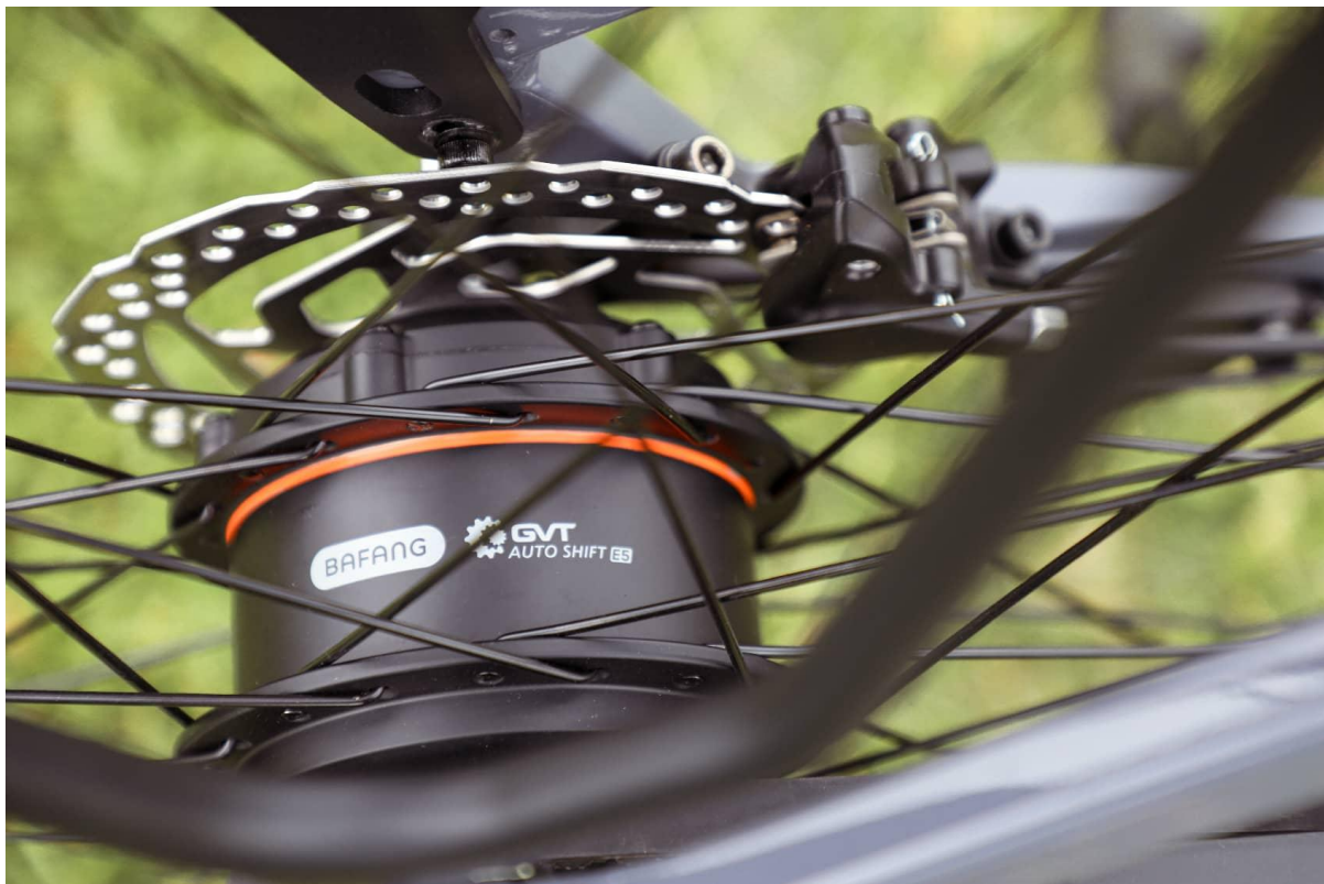
Figure 1 - Bafang RG E510 5-speed auto & manual electronic gear hub
