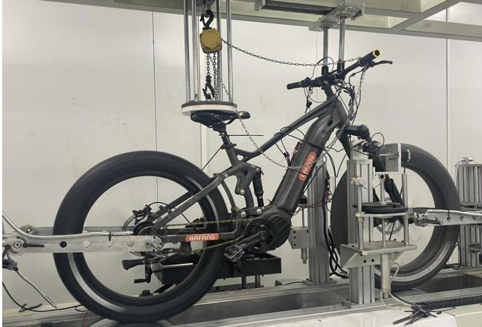
*Photo: G500A simulated load testing*
