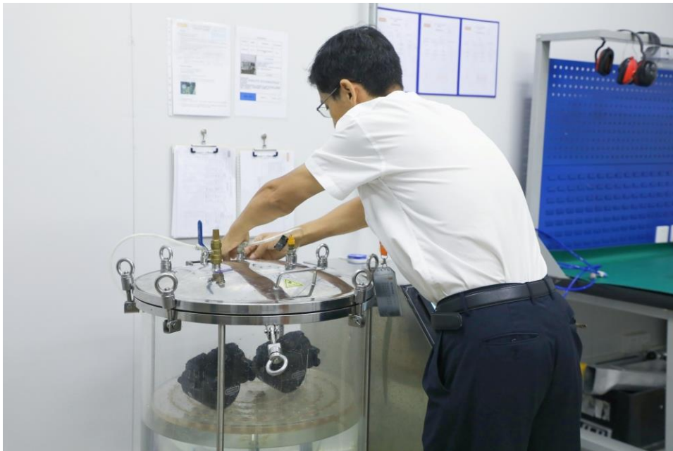
Photo: An engineer operating the air tightness tester
