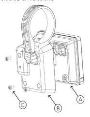
Open the clamps of display and place the display on to the handlebar in the correct position. Now with M3\*14 screws (A) tighten the display into position. Torque requirement: 0.3N.m.
