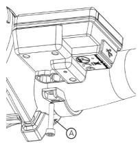
Open the clamps of controller panel and place it on to the handlebar in the correct position. Now with M4\*12 screws (A) tighten the controller panel onto position. Torque requirement: 1N.m.
