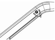
3. Then using the lever, push the lever up to release the second locking mechanism.
