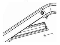
2. Now push the top part of the battery into the frame, until you hear the battery lock into position, and the battery cover sits flush with the frame.
